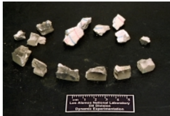
Figure A-6. PBX 9501 fragments retrieved from the firing mound from test K8-2171. Each of the violent reaction tests resulted in HE dispersal on the firing mound.
